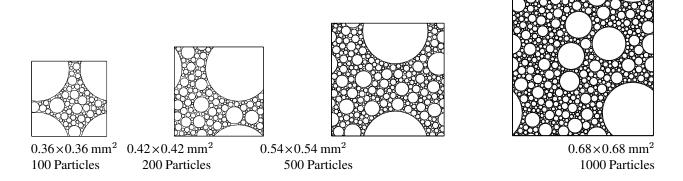
Figure 9: Circular particle models based on the particle size distribution of pressed PBX 9501.
