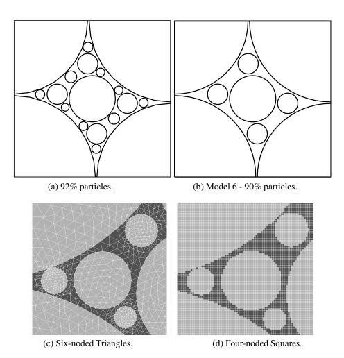
Figure 7: Microstructure containing 92% particles modeled with six-noded triangles and four-noded squares.
