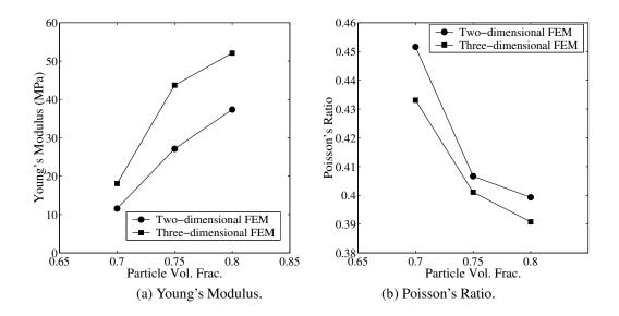
Figure 4: Two- and three-dimensional estimates of effective Young's modulus and Poisson's ratio.
