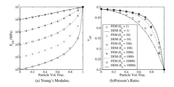
Figure 2: Comparison of finite element (FEM) and differential effective medium (DEM) predictions.  $E_b$  is the Young's modulus of the binder.
