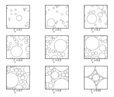
Figure 1: RVEs containing 10% to 92% by volume of circular particles.  $f_p$  is the volume fraction of particles in a RVE.
