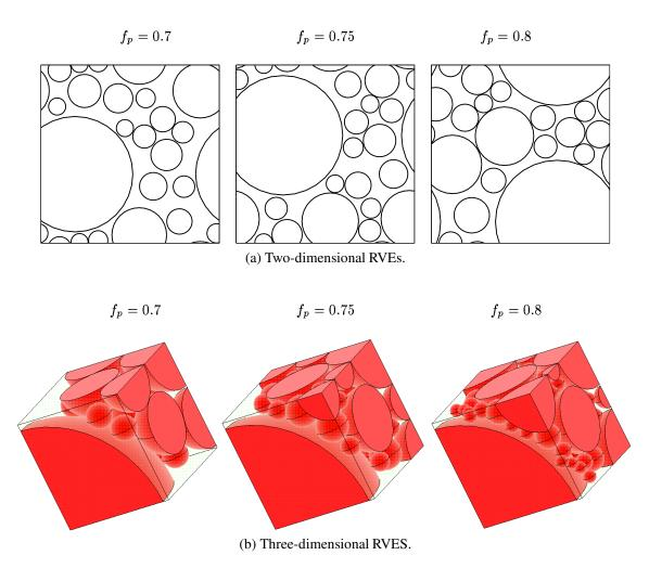
Figure 3: Two- and three-dimensional RVEs containing 70%, 75% and 80% particles by volume.  $f_p$  is the volume fraction of particles.
